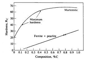
We may note that hardenability is not "hardness", which is the resistance to indentation; rather, hardenability is a qualitative measure of the rate at which hardness drops off with distance into the interior of a specimen as a result of diminished martensite content
