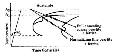
The increase in cooling rate due to air cooling as compared with furnace cooling affects the transformation of austenite. There will be less *proeutectoid* ferrite in normalized hypo eutectoid steels and less pro eutectoid cementite in *hypereutectoid* steels as compared with annealed ones. Since it was cementite network which reduced the strength of annealed hypereutectoid steels, normalized steels should show an increase in strength.
