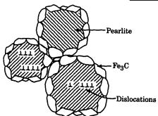
Full annealing is used to refine the grain of large steel castings and forgings to give improved ductility and strength.
