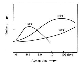
Hardness is a measure of the strength of the alloy. Obviously, the maximum hardness and strength is obtained only for the right combination of temperature and time. This combination is a function of the copper content and the other impurities in aluminium.
