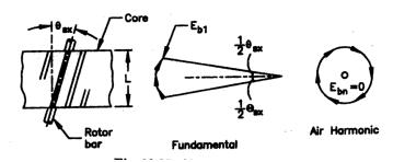
If either stator or rotor slots are skewed, the variations in flux density, magnetic pull, and torque due to the slot openings will be displaced in time phase along the core length, resulting in more uniform torque, less noise, and better voltage waveform. In order to eliminate the effect of any harmonic, the rotor bars should be *skewed* through an angle so that the bars lie under alternate harmonic poles of the same polarity or in other words, bars must be skewed through two pitches.
